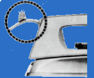
Insulation break down due to Fatigue.
